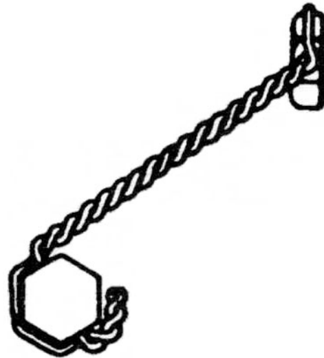
Figure 6: Wiring perpendicular fasteners.
