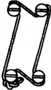
Figure 7: The single wire method used on closely spaced fasteners.
