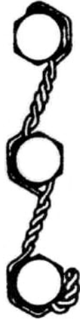
Figure 2: Note that in the double twist method, the wire is twisted in alternating directions between pairs of fasteners.
